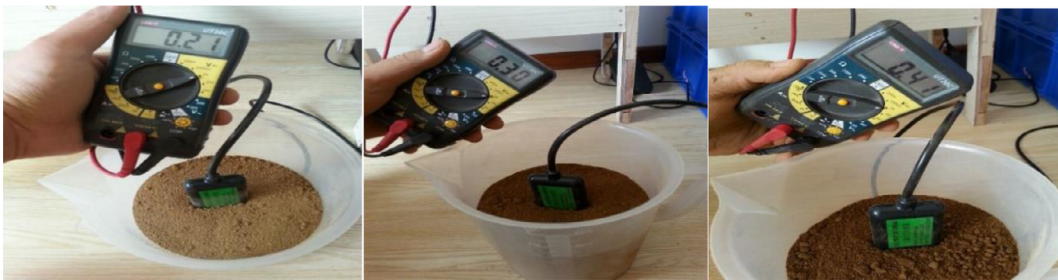
Fig. 3. Soil moisture changes after adding 100 ml of water each time.
